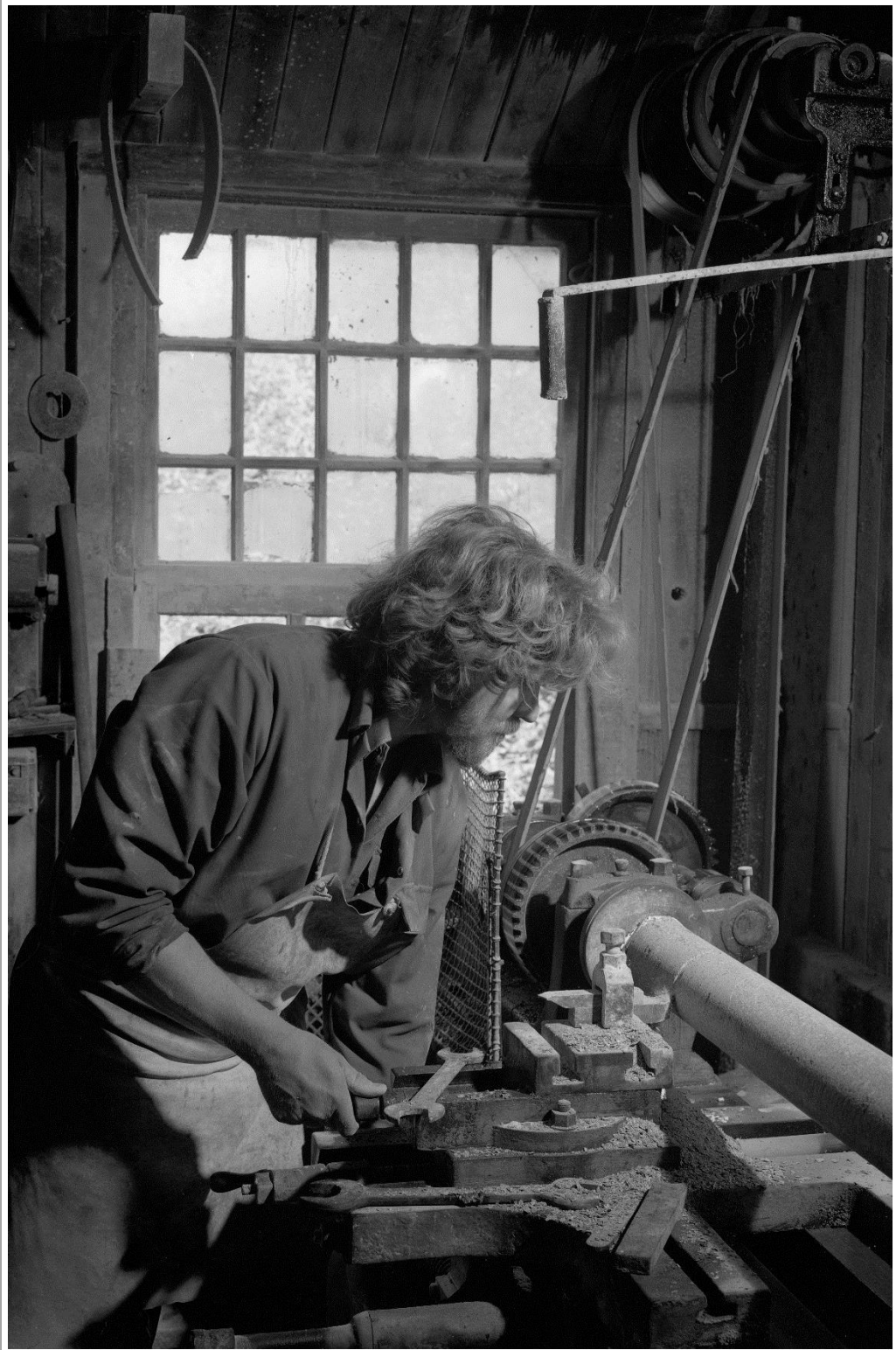
Brian Bugler lathe turning Purbeck Marble - St Aldhelm's Quarry.
